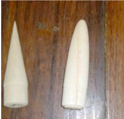
Patrick's nosecones. Extra mass was added to the payload of the pointed and elliptical cones so that each rocket had the same mass.
