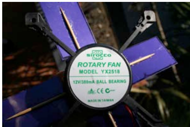
Buy a fan and run it backwards as a generator.
