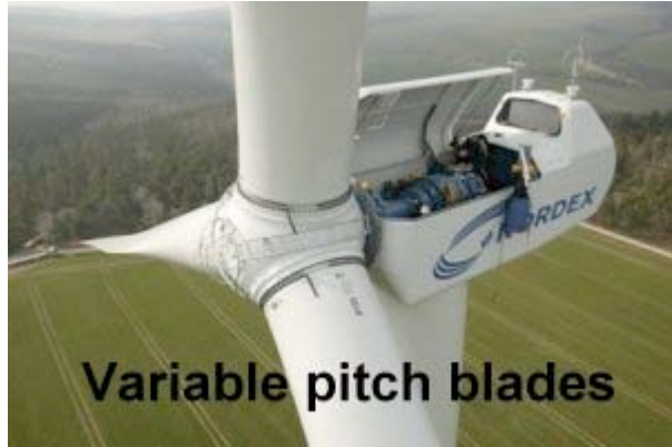
Variable pitch blades Need to decrease the pitch in high winds or else.
