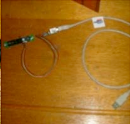
The altimeter's data can be downloaded via a USB connection and analysed for altitude, acceleration and velocity of rocket flight. More photos from Patrick's EEI can be seen here.
