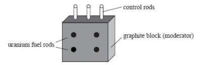
The function of the moderator is to slow down the neutrons produced in a reaction such as that described above.
