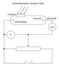
The potential difference V applied between the metal plate and electrode may be varied in magnitude and in direction. This is repeated for different values of intensity for the same frequency of light.
